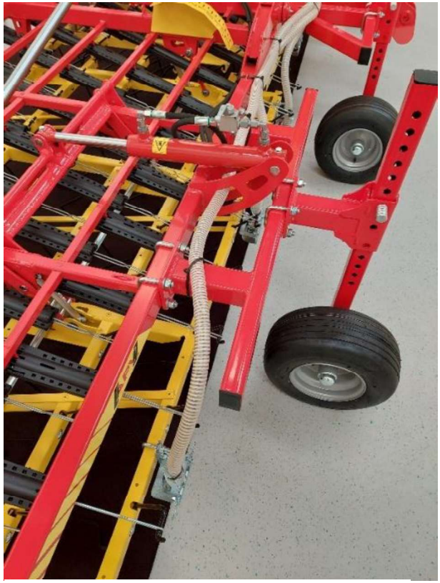
Figure 70: Hose laying along the harrow 6
