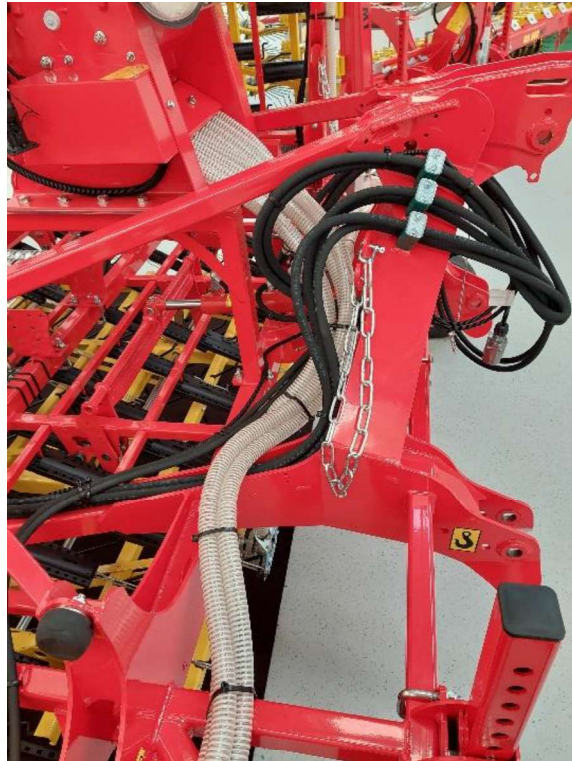
Figure 65: Hose laying along the harrow 1
