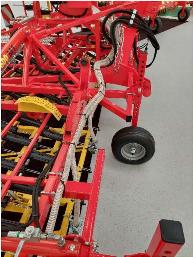
Figure 69: Hose laying along the harrow 5
