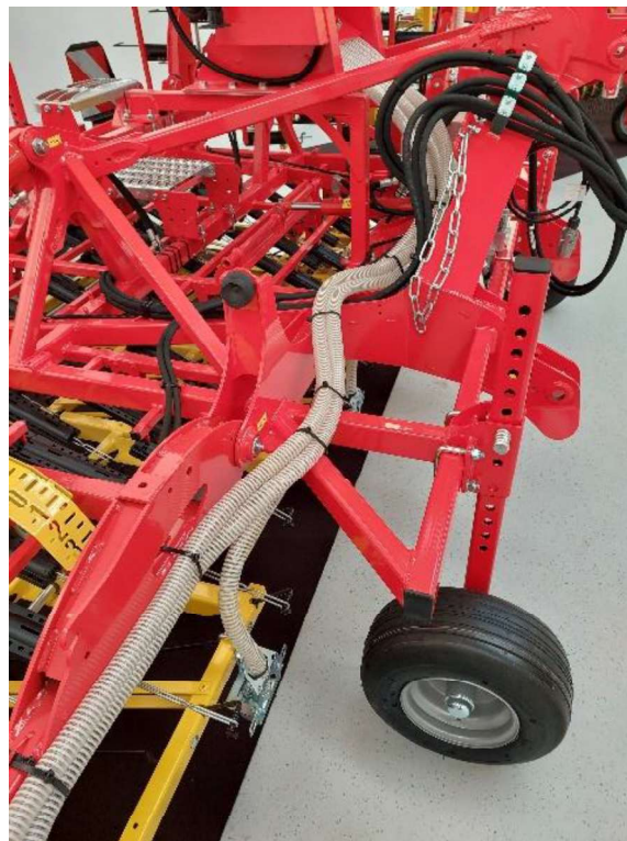
Figure 66: Hose laying along the harrow 2
