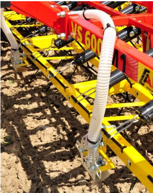
Figure 74: Hose laying along the harrow 10
