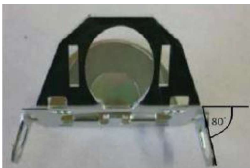
Figure 41: Bending the lateral dispersion plates
