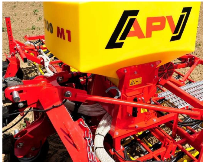
Figure 61: Hose laying starting from the PS outwards 1
