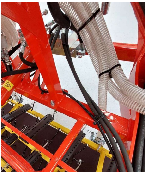
Figure 64: Hoses to the dispersion plates on centre frame 2
