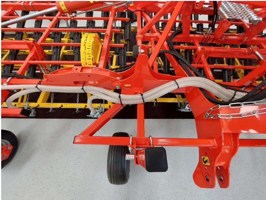
Figure 67: Hose laying along the harrow 3
