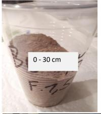
Weigh exactly 100 grams of the sieved soil in the cup (visible on the image: 0 - 30 cm soil depth and previously determined factor 1.5)
